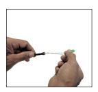
Step 4: Prepare the connector Clamp the fibres and pull the mesh back. Ready to connect to the adapters
